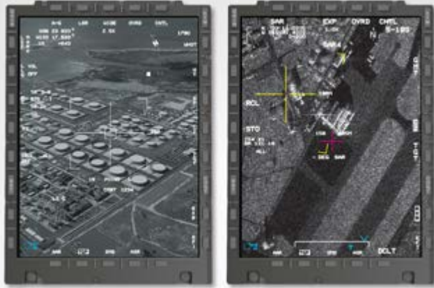
2. Right Photo: Center Pedestal Display, Targeting and SAR Imagery
