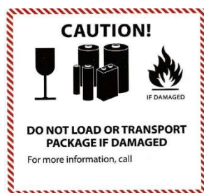
Lithium Battery Label
