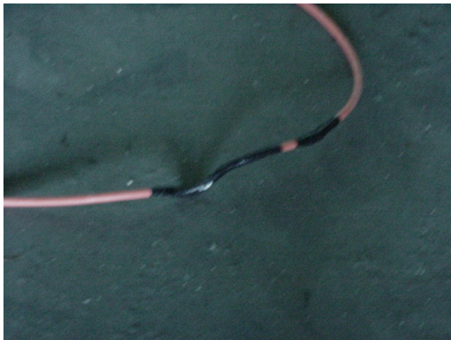
Tape on Cord Set Go to "Table of Contents"
